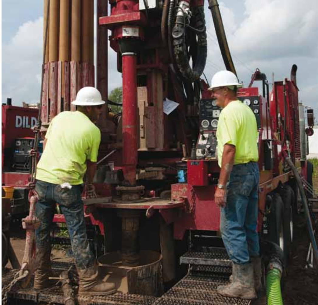
*(above) The rig is quiet enough even while drilling, owner-driller Wayne Findlay and helper Mike McCall can easily communicate over rig's single 500 hp engine.*
